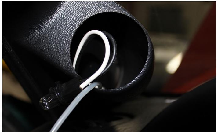
6. Connect the vacuum line and bulb to the gauge, then mount the boost gauge. For one of our gauge pods, simply press it into place - no hardware is necessary to secure it. If the studs in the back of the gauge interfere, cut them off. Don’t use a saw that will vibrate, as that can cause damage to the gauge. Instead, use side cutters that will pinch it off. If you’re mounting it elsewhere, do that now. That’s it, you’re done!
