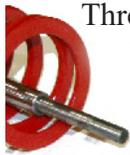
Thread the spring perch down to allow you to more easily install the shock mount - because of the adjustable spring perch, no spring compressor is necessary for installation of this setup.
