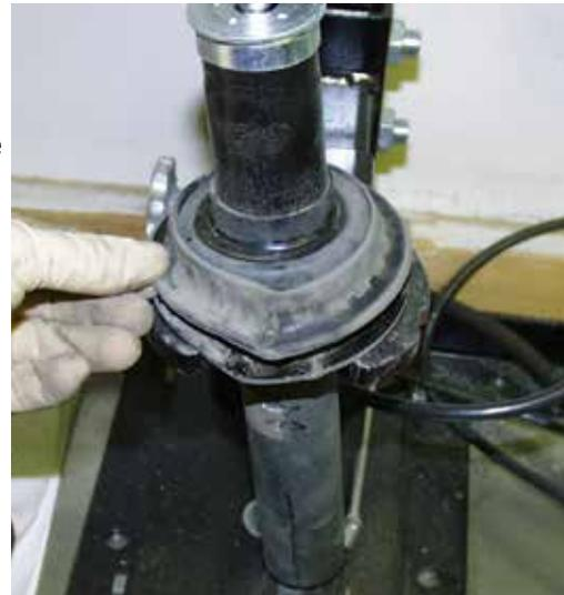
We don't recommend the use of these springs with stock shock absorbers. The stock shocks do not have the damping required to control a stiffer spring and will give lousy performance and ride quality. If you're using our Tokico Illumina shocks, we suggest starting with the damping set to 3 in the front and 2 in the rear. Please note that these are not pre-set.
