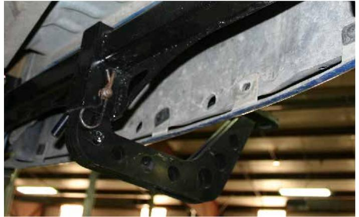
**Receiver Hitch Attachment only:** There is an additional hole at the top of the hitch (4) to eliminate the typical hitch wobble. You'll run the included bolt through the hole and tighten it down. You don't *have* to use this, but it is suggested. That's it, you're done. Now go tow something!
