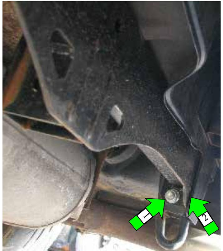
3. Press the hitch back into place. Slip all of the bolts through the holes before you tighten any of them. Use the “nutplates” for the upper bolts on both sides (3). Once all of the bolts are in place with nuts, tighten them all. Be sure to use a washer under the bolt head and the lower nut. The upper nut with the nutplate needs one under the bolt head but not under the nut.
