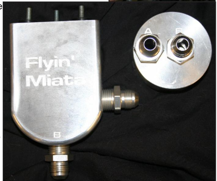
8. Now it's time to play with the filter mount. If you're feeding your turbo off of the filter mount, you should install a 1/8NPT to AN adapter (not included) in the third, smaller hole. The stainless turbo feed hose will go to this adapter. Otherwise, you can tighten the pre-installed plug or install some type of fluid sender, if you have one. If you're using a sender, you'll probably want to install that once the mount has been installed.
