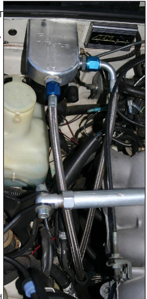
on the fitting - or, of course, the ubiquitous adjustable wrench. If you're picky about appearances, protect the aluminum somehow - it's easy to knick the anodizing. Tighten them down, but don't over-tighten them, which is a common mistake. They should be torqued to 29 ft-lbs, or hand tight plus a quarter-turn. If you're curious, oil flows into the side of the filter from the "A" hose, through the middle of the filter and out through the "B" hose.
