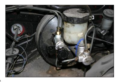
you're tightening the stock fitting, to ensure that nothing is damaged. Again, no Teflon tape.
