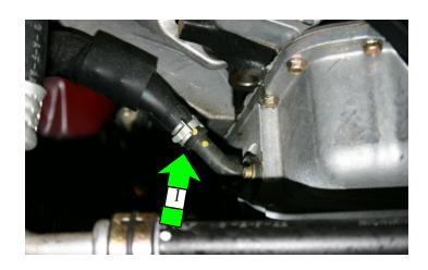
2. Trim 3/4" from the large hose (2), at the end indicated by the arrow. Then trim 1/4" from the tapered hose (3), again at the end indicated by the arrow. The new hose is used to connect the bottom half of the check valve to the fitting in the oil pan.
