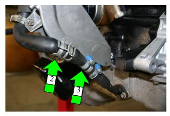
3. Slip the check valve into the new hose, being sure that fluid can flow into the pan but not up from the pan (arrow #4 should point up, away from the pan). Snug the hose clamps and you're done!
